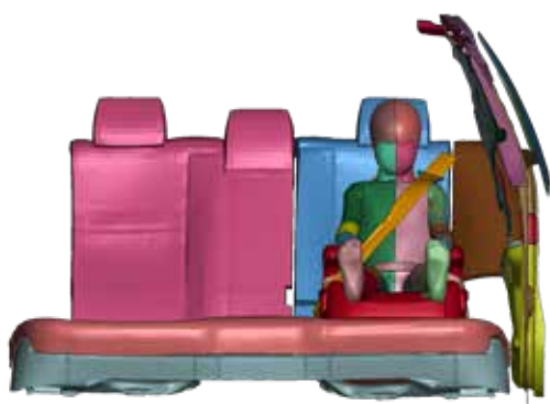
Simulation of a child passenger in a car seat before a side impact collision (left) and during collision
