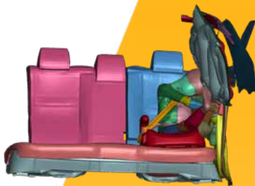
Simulation of a child passenger in a car seat before a side impact collision (left) and during collision
