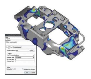
With PTC Creo Fatigue Advisor Extension, you can easily estimate the number of load cycles your model can sustain before failure.
