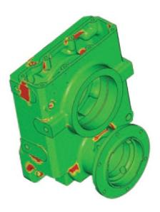
With the confidence of life plot, you can quickly examine the ratio between the calculated life and the target design life.
